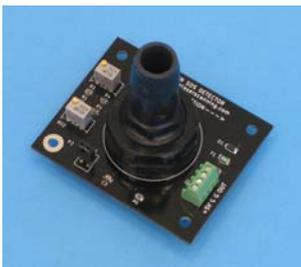
The PRECISION SOS DETECTOR™ is the first commercially available Start-Of-Scan detector made for the challenging environment inside a high power Polygon Scan Head. It is designed to work with the PRECISION SOS LASER DIODE MODULE™
