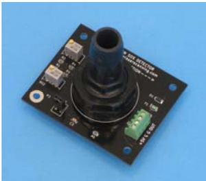
An SOS detector is required to achieve accurate line to line registration with any polygon scanner. It is used to synchronize a CW or pulsed laser to the scanner. (Galvo scanners need absolute encoders, polygon scanners need Start-Of-Scan detection.) Read more about it here:
